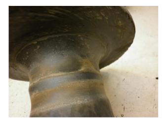
The roll has flat spots caused by blockade.
