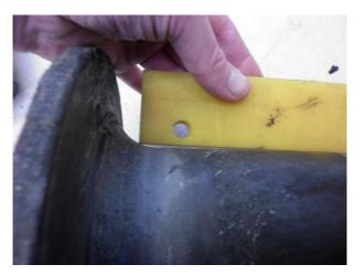
Wear is about 1mm, the roll are used for some time. Normally maintenance, inspection on rope.
