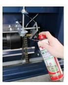
Clean chains, gears and rolls and remove run-in ropes and leaves (when necessary). If necessary, tighten the chain by turning the mounting-nut from the engine (located behind cover underneath control panel. Do not over-tighten the chain, the minimal sideways tolerance should be approx. 1 cm. Once the correct chain tension has been achieved, retighten the mounting-nut with the contra nut.
