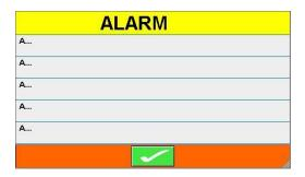
A failure can interrupt the automatic program and the cause of the failure will be showed on the screen. For resetting the failures press the button.
