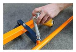
The pivot points of the next items must be oiled when necessary but at least twice a year: Safety bumper, flag/fin, lock pins, Wheel bearings, and reel chain.
