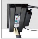
Perform an equalisation charge. MIDAC MIDATRON battery chargers automatically equalise the battery at the normal completion of the recharging cycle. Other brands and/or older chargers may require you to manually start equalisation.
