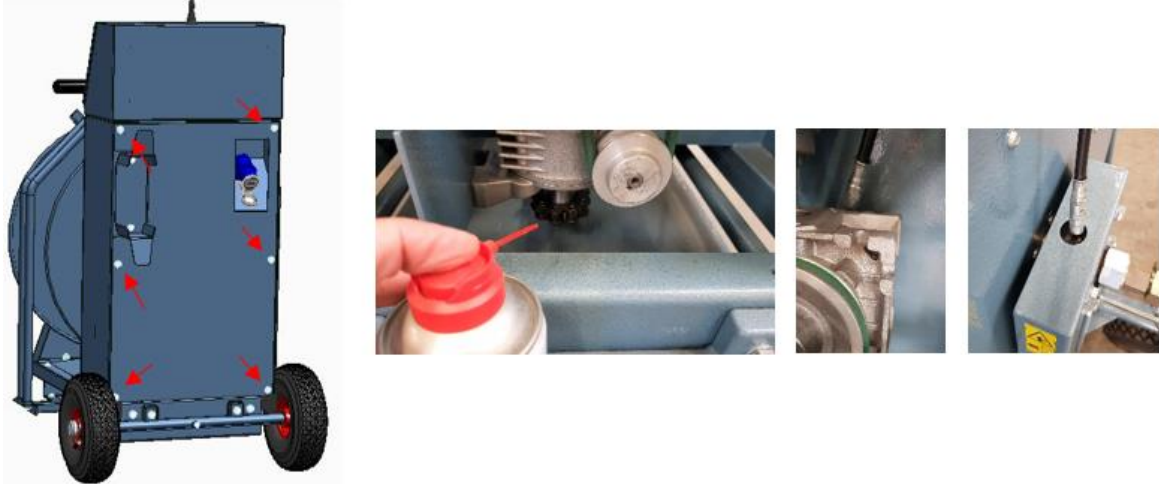
Figure 9.4; Greasing the chain guide and drum bearings
