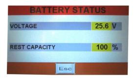
The screen shows the battery voltage in Volts and gives an indication of the remaining capacity in %.
