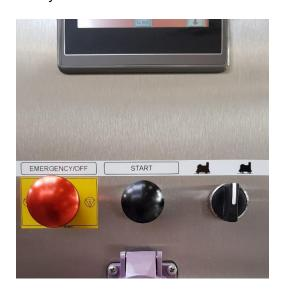
Turn the knob to the right to activate the lifting system. Move the *METO* and turn the knob to the left to let the lifting system go in completely until a beep is heard.
