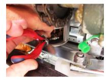
1) Blow the engine clean with (dry) air. 2) release the brush spring 3) and pull the brush at the wire from the holder.
