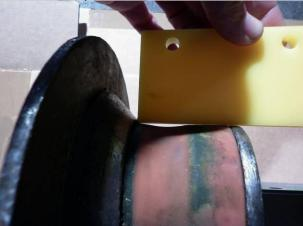
Wear is about 1mm, the roll are used for some time. Normally maintenance, inspection on rope and grease the chain and when necessary tension the chain.
