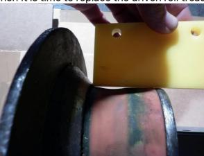
Wear is about 1mm, the roll are used for some time. Normally maintenance, inspection on rope and grease the chain and when necessary tension the chain.
