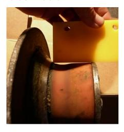
Wear is 2 – 3 mm, the roll is still good. Normally maintenance, inspection on rope and grease the chain and when necessary tension the chain.
