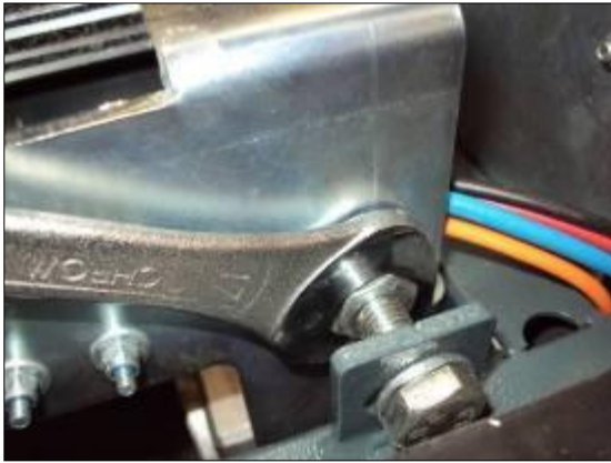
Figure 6: Unscrewing / tightening locking nut
