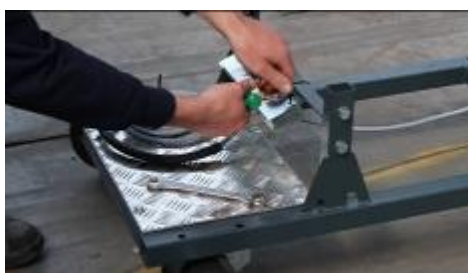
Release the control box
