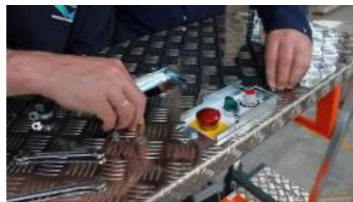
position the control box and screw it down
