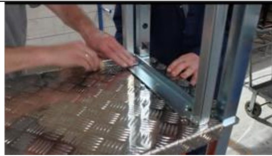
secure the rail with the bolts
