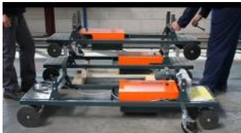
De-stack the EasyKits removing the casings
