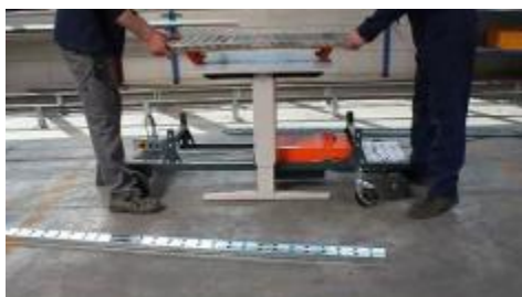
Put the platform onto the bench
