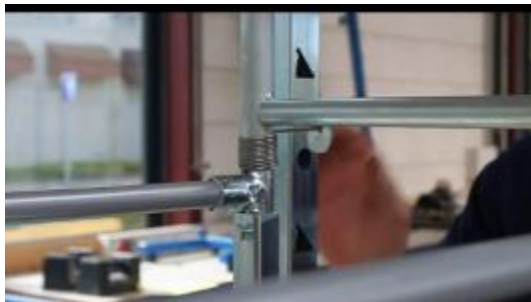
Fit the safety rail spring
