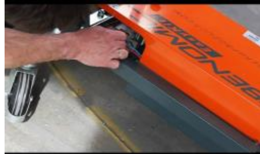
put the supply plug into the connector
