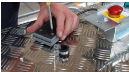
Remove the bolts from the foot switch
