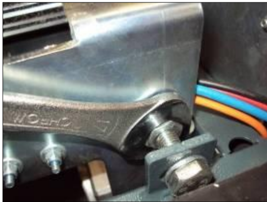
Figure 6: Unscrewing / tightening locking nut
