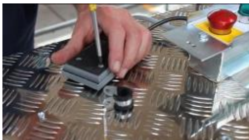
Remove the bolts from the foot switch
