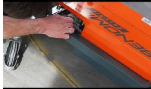
put the supply plug into the connector
