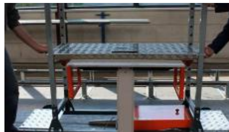
now slide the remaining poles into the holes
