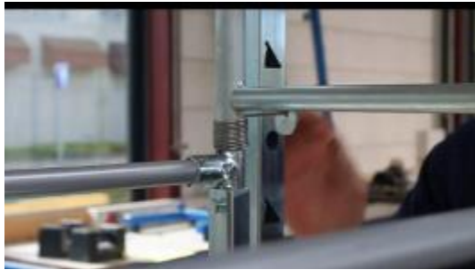
Fit the safety rail spring
