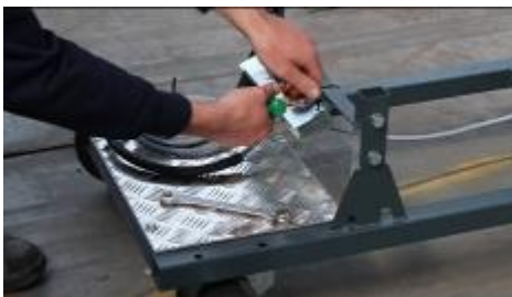
Release the control box
