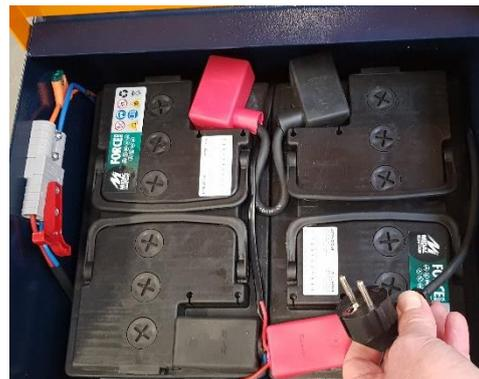
**Charge the batteries according to the status of the battery condition meter when they have between 50% and 20% remaining capacity, but try to do this as often as possible when the status is around 20% in accordance with the following recommendations.**
