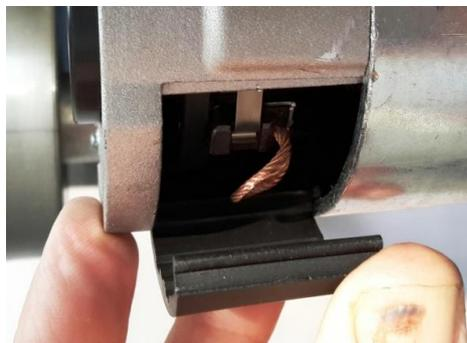
Figure 5: Inspecting the carbon brushes
