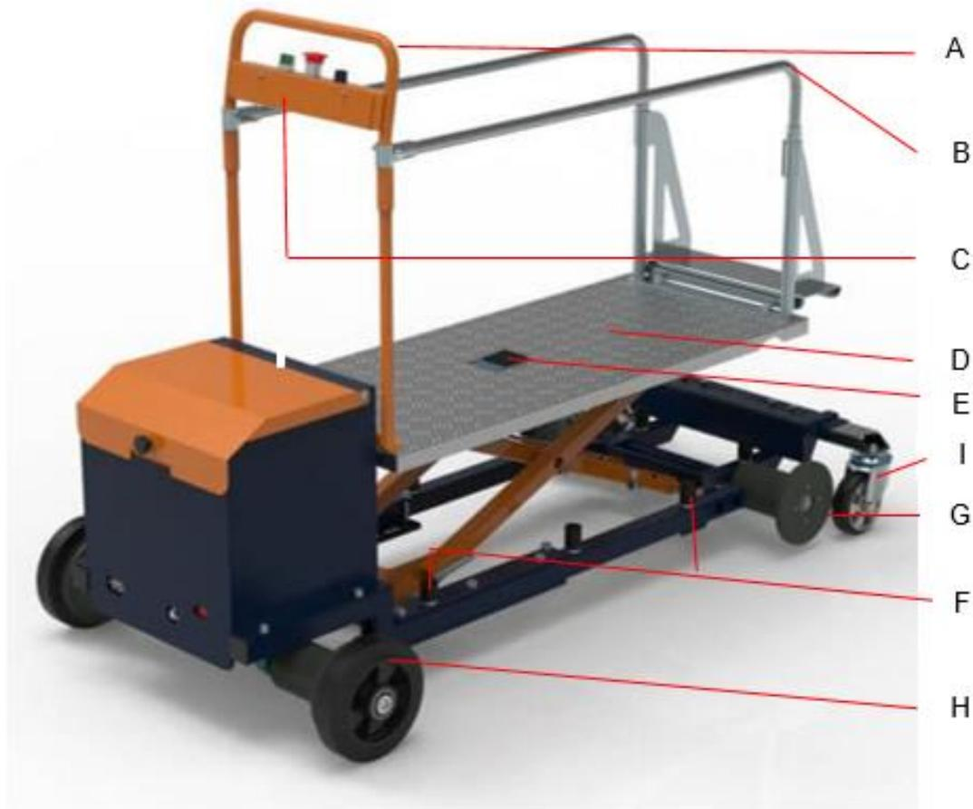
Figure 1: Principal components of the *Leaf picking cart*
