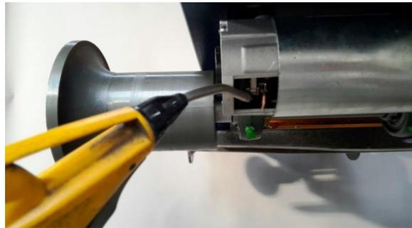
Dismantle the black plastic cover and blow the motor clean using (dry) compressed air.
