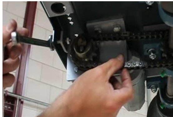
Figure 7: Tensioning the chain
