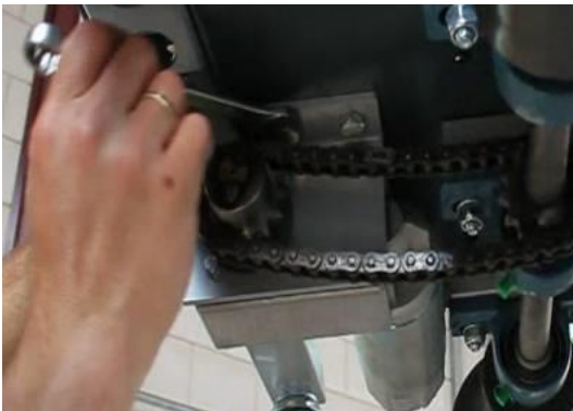
Figure 6: Unscrewing/tightening the motor bolt
