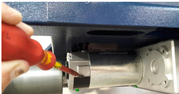
Figure 5a: Cleaning the carbon brushes
