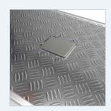
Because the foot pedal comes flush with the level of the platform, this increases the ergonomic posture for the employee.
