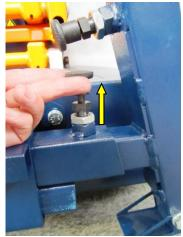
Fig. 2. Release locking pin
