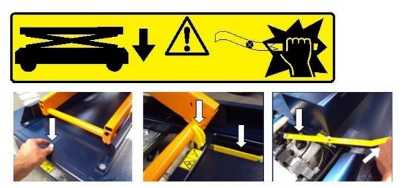
Fig. 6.5 - Left: unscrew bolt and remove cover. Centre - take out the handle. Right - press the bolt in the gap against the pin on the emergency lowering valve!
