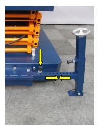
Fig. 4. Locked stabilizer arm
