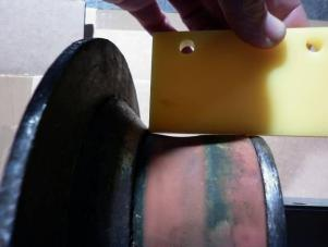
Wear is about 1mm, the roll are used for some time.
