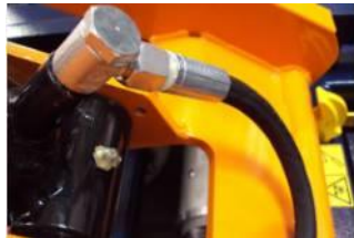
Figure 9.3; Location of the grease nipples at the cylinder
