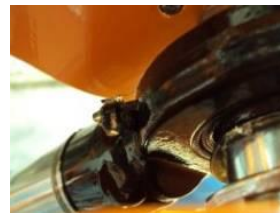
Figure 9.3; Location of the grease nipples at the cylinder
