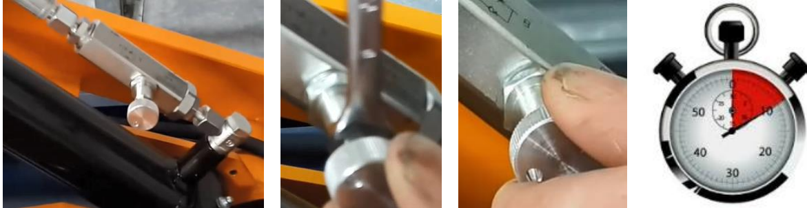
Figure 9.6: Adjusting scissors platform fall velocity
