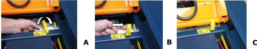
Figure 9.1 A-B-C; Unlocking the scissor blocks
