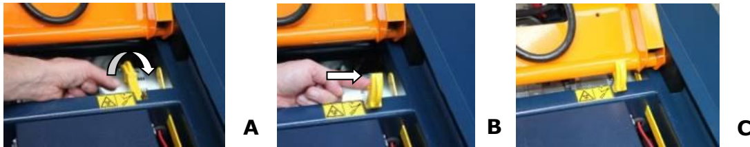
Figure 9.1 A-B-C; Unlocking the scissor blocks
