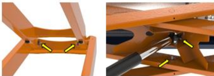
Figure 9.2; Location of the grease nipples for the scissor and cylinder shafts
