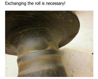
The roll has flat spots caused by blockade.
