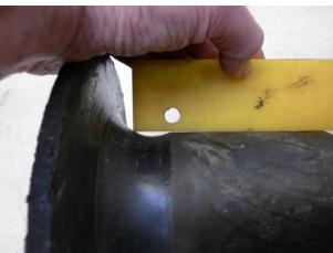
Wear is 2 – 4 mm, the roll is still good. Normally maintenance, inspection on rope. To change the roll is not necessary, do not create unnecessary cost!
