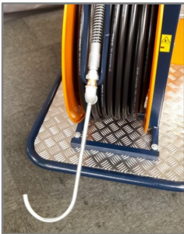
Figure 7.2: Assembly of the pipe hook
