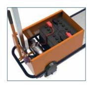
Thanks to the electronic motor control in combination with strong traction batteries, sufficient power is also available at low speeds and for a longer period.
