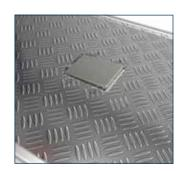
Because the foot pedal comes flush with the level of the platform, this increases the ergonomic posture for the employee
