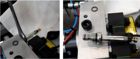
Step 6: Blow with air pressure the dirt out of the valve, push on the button so that the valve is switched open.
