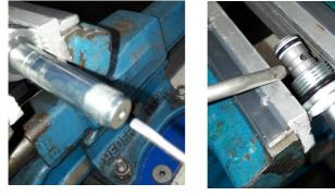
After this the valve should be cleaned, and can be installed again, so you can check if the problem is solved.
