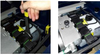
Step 5: Take out the valve from the pump-unit (tool size 24)
