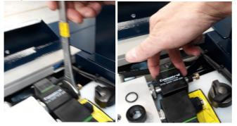
Step 5: Take out the valve from the pump-unit (tool size 24)
