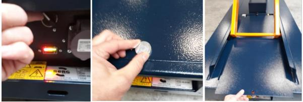
Step 2: Turn up the yellow safety scissor block. After this you can lower the scissors until it hits the yellow safety scissor block.
