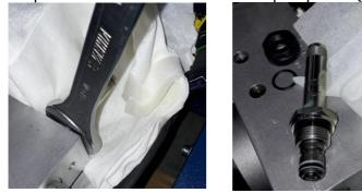
Step 6: Blow with air pressure the dirt out of the valve, please push careful with a screwdriver into the end of the valve, which will open the valve.
