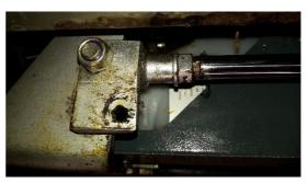
Step 4: Install the mounting bracket from the defective gas spring to the new one and mount the gas spring.
