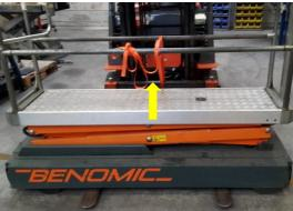
Step 2: Make sure that the forklift paddles are sufficiently crossed and lift the Benomic under the lifting wheels as shown.
