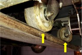
Step 3: Remove the gas spring as shown, make sure that only **nut A** is loosened, **nut B** must keep the same position!
