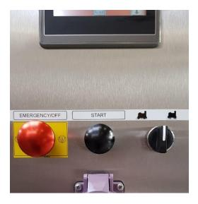
Turn the knob to the right to activate the lifting system.
