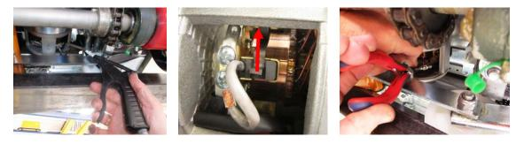
1) Blow the engine clean with (dry) air. 2) release the brush spring 3) and pull the brush at the wire from the holder.
