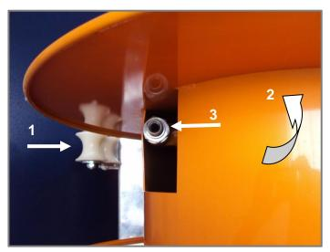
Figure 7.2; Order in which the hose should be mounted to the reel
