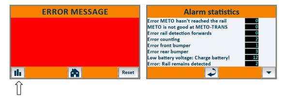
The previous failures are shown on the alarms screen by pressing the statistic button.
