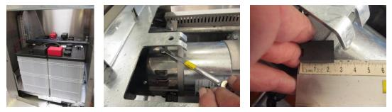
Put the *BeMatic Meto SW* down carefully to the ground, remove the batteries and repeat the above operations for the two brushes at the top of the engine.
