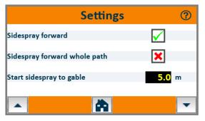
[SIDESPRAY FORWARD WHOLE PATH] This setting is active as standard so that the entire path is sprayed.
