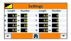
[PATH LENGTH: SECTION A (to Z)] Enter the length of the paths per section.
