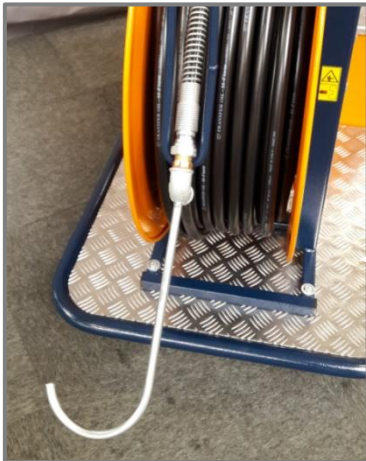
Figure 7.2: Assembly of the pipe hook
