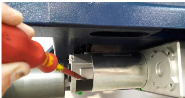
Figure 5a: Cleaning the carbon brushes
