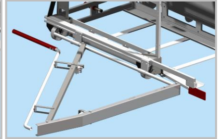
Figure 7.3; MetoTrans with guide arm and detection fin
