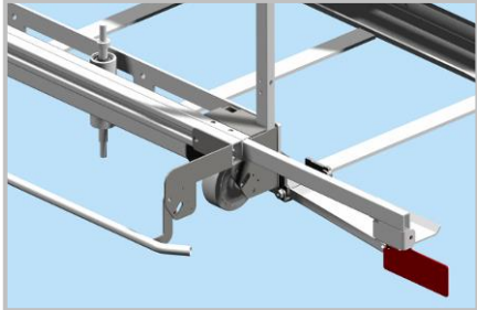
Figure 7.1 MetoTrans with pin guide, safety bumper and detection fin
