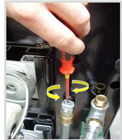
Figure 7.4; Adjusting the pressure switch
