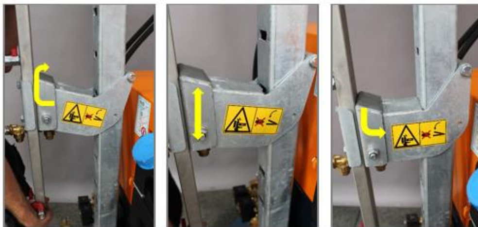
Figure 7.2: Adjusting the spray boom
